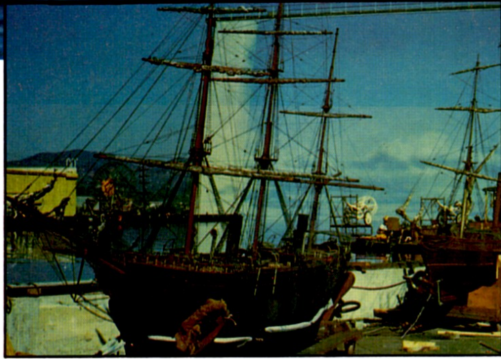
An effects crew rigs the model of the nitrate ship at Fox's Sersen tank. The free-floating model was designed to be pulled through the water by cables. Inset: The Abraham Lincoln and nitrate ship miniatures in their storage carriers.
